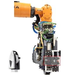
Leica AT960 laser tracker and drilling end effector with mounted T-Mac (highlighted)
