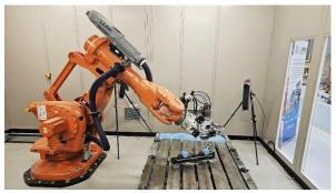
Robotic milling platform with IONA photogrammetry system
