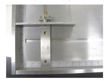
Figure 2: Vertical slide calibration check
