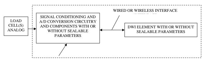
If NTEP Certification is for the signal conditioning element and the DWI element (the whole weight indicating element), use the Digital Electronic Scales (DES) examination procedure.
