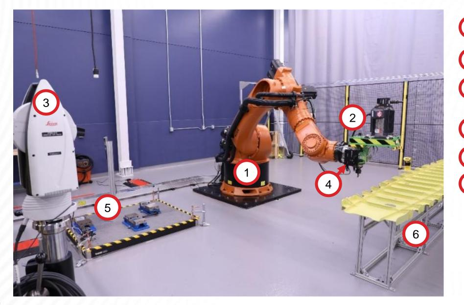
1 KUKA KR500-3 Robot Mill 2 Leica AT960 3 Laser Tracker Leica T-Mac 4 Tracker Target 5 Vices Wing rib 6
