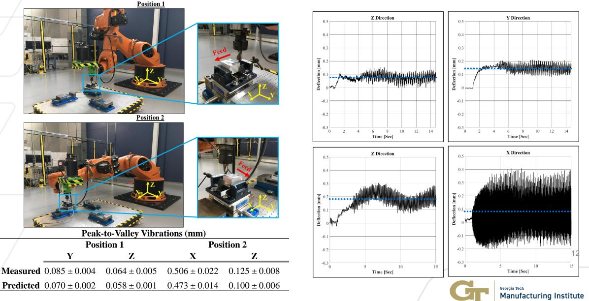
The GPR model peak-to-valley vibration predictions are correlated to the measured behavior
