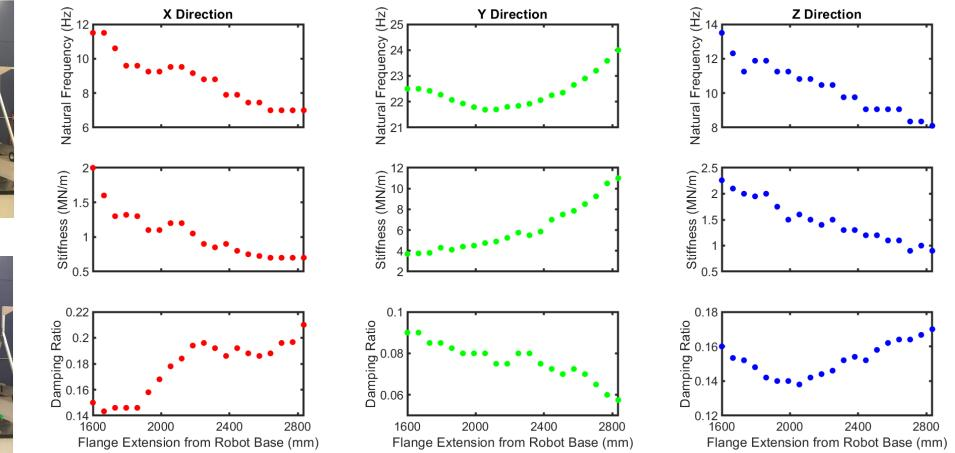
The data shows that the modal parameters change with arm configuration, and therefore arm configuration must be considered in controller tuning<sup>Manufacturing Institute</sup>
