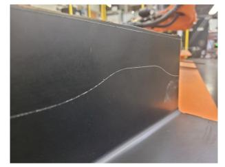
CFRP part with Scribe Line
