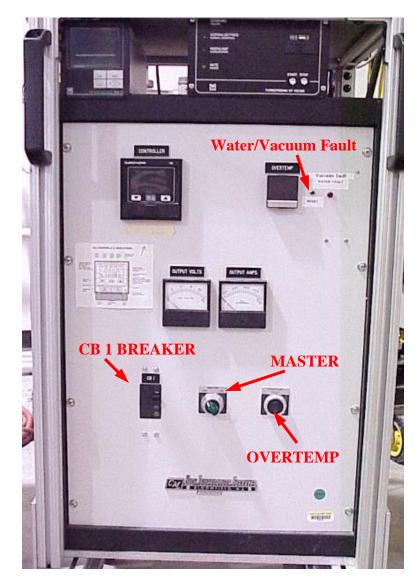
**Figure 2. Furnace power cabinet**
