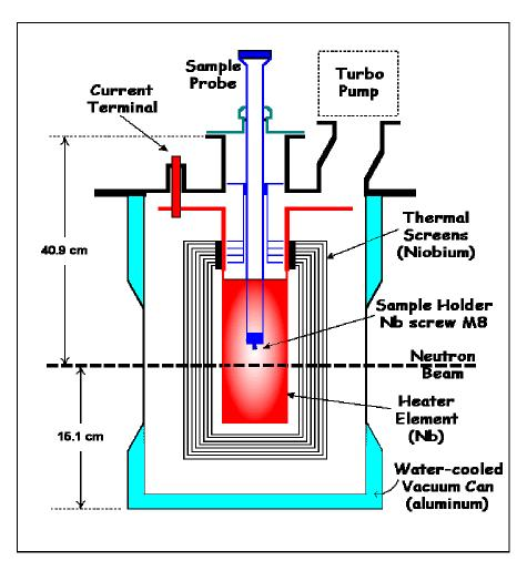
Figure 1. AS1600 C Furnace body cross section schematics
