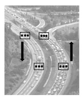
**Figure 6:** Traffic zones are an aggregation of traffic lanes. The dots are traffic lane detectors and the boxes are the traffic zones. In this figure, there are 12 traffic lane detectors: 4 traffic zones with 3 detectors in each zone. There is one traffic zone detector per road segment in each direction. In the data, there are different numbers of lane detectors in each traffic zone. This photo was obtained from National Archives [6].
