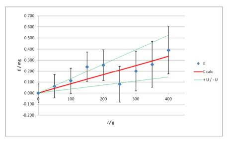
The residuals and the uncertainties associated with the calibration points are calculated by (C2.2-7) and (C2.2-11) respectively, and are shown in Table H4.6.
