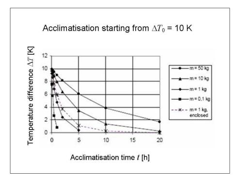
Tables F1.2 and F1.3 give acclimatisation times  $\Delta t$  for standard weights that may have to be waited if the temperature difference is to be reduced from a value  $\Delta T_1$  to a lower value  $\Delta T_2$ . The conditions of heat exchange are the same as in Figure F1.1: Table F1.2 as for "m = 0,1 kg" to "m = 50 kg"; Table F1.3 as for "m = 1 kg enclosed".
