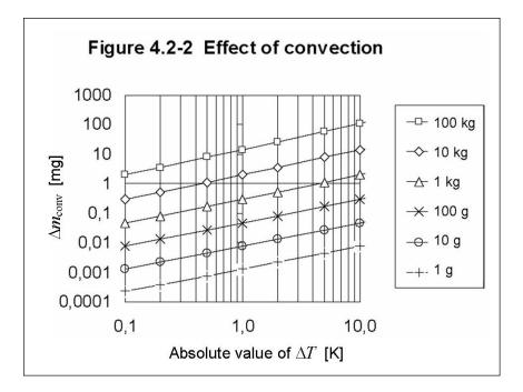
Figure 4.2-2 gives an impression of the magnitude of the apparent change in mass in relation to a temperature difference, for some selected weight values.
