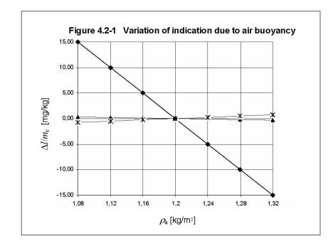
Line  $\blacktriangle$  is valid for a body of  $\rho = 7\,810 \text{ kg/m}^3$ , weighed in  $\rho_a = \rho_{as}$  (as for case c above) Line  $\bigstar$  is valid for a body of  $\rho = 8\,400 \text{ kg/m}^3$ , weighed in  $\rho_a = \rho_{as}$  (as for case c above) Line  $\blacklozenge$  is valid for a body of  $\rho = \rho_s = \rho_c$  after adjustment in  $\rho_{as} = \rho_0$  (as for case b above)
