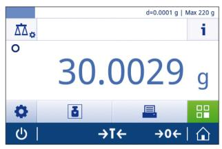
After a short period of time, the weighing pan is stable. The unstability symbol • disappears and the value in the weighing value field becomes dark blue again.
