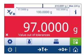
In the example below, the defined target weight is still 100.000 g and the tolerance limit is  $\pm 2.5$  %. The sample weight is 99.0000 g.
