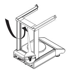
Push the lock button to release the rear glass.
