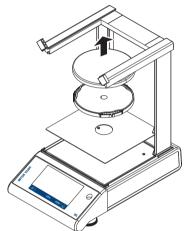
Remove weighing pan, pan support and bottom plate.
