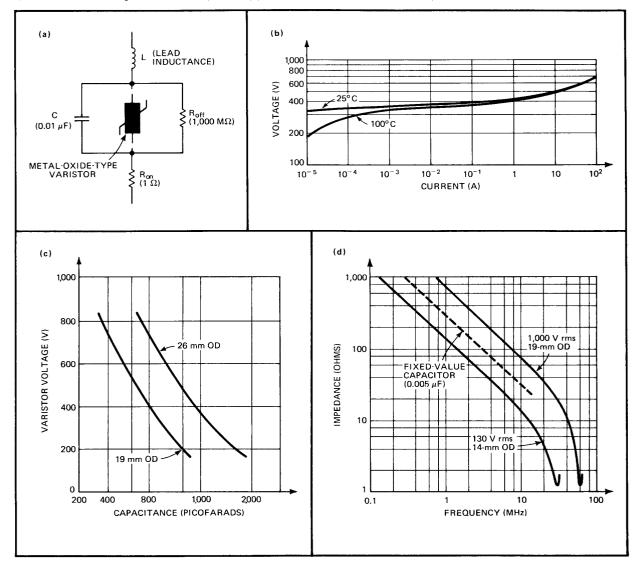
one with a 130-V rms rating, and the other with a 1,000-V rms rating. A point-of-reference curve for a fixed 0.005-microfarad capacitor is also included.
