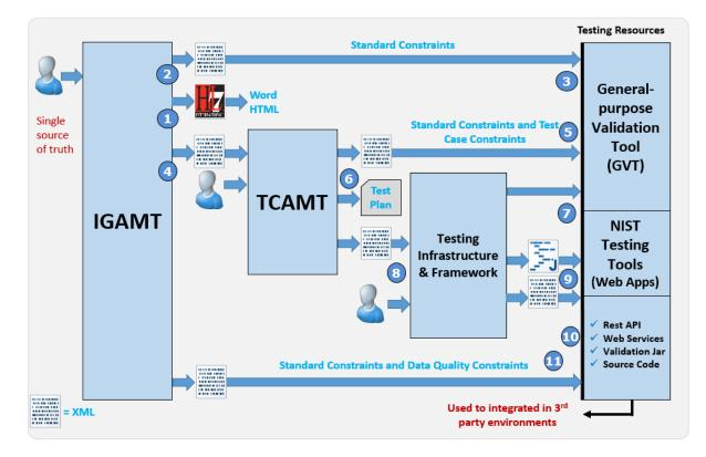
Figure 3: NIST HL7 v2 Standards Development and Testing Platform Architecture
