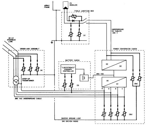
Figure 3-3. Overvoltage protection at system interfaces
