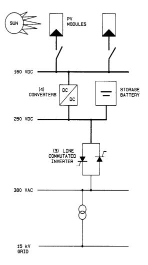
Figure 3-1. Block diagram of the Kythnos photovoltaic system
