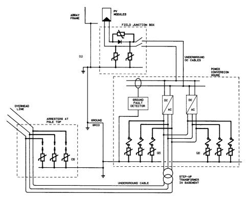
Figure 2-2. Surge protective devices at system interfaces
