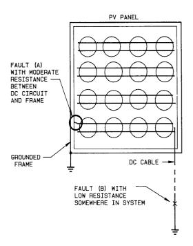
Figure 2-4. Scenario of double ground fault
