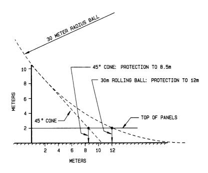
Figure 3-6. Cone-of-protection and rolling-ball criteria
