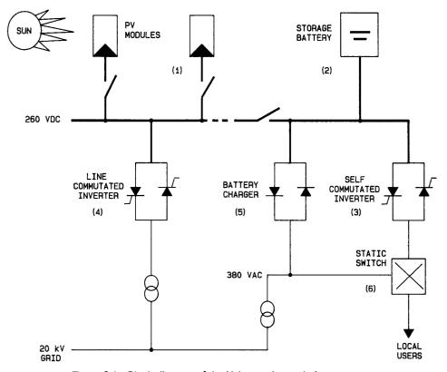
Figure 2-1. Block diagram of the Vulcano photovoltaic system
