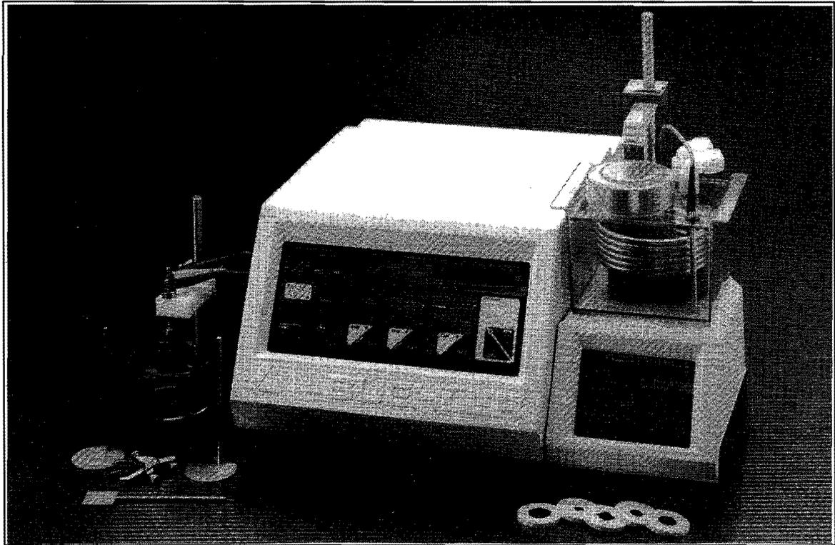
Figure 1. ELECTROMET® 4 Polisher/Etcher
