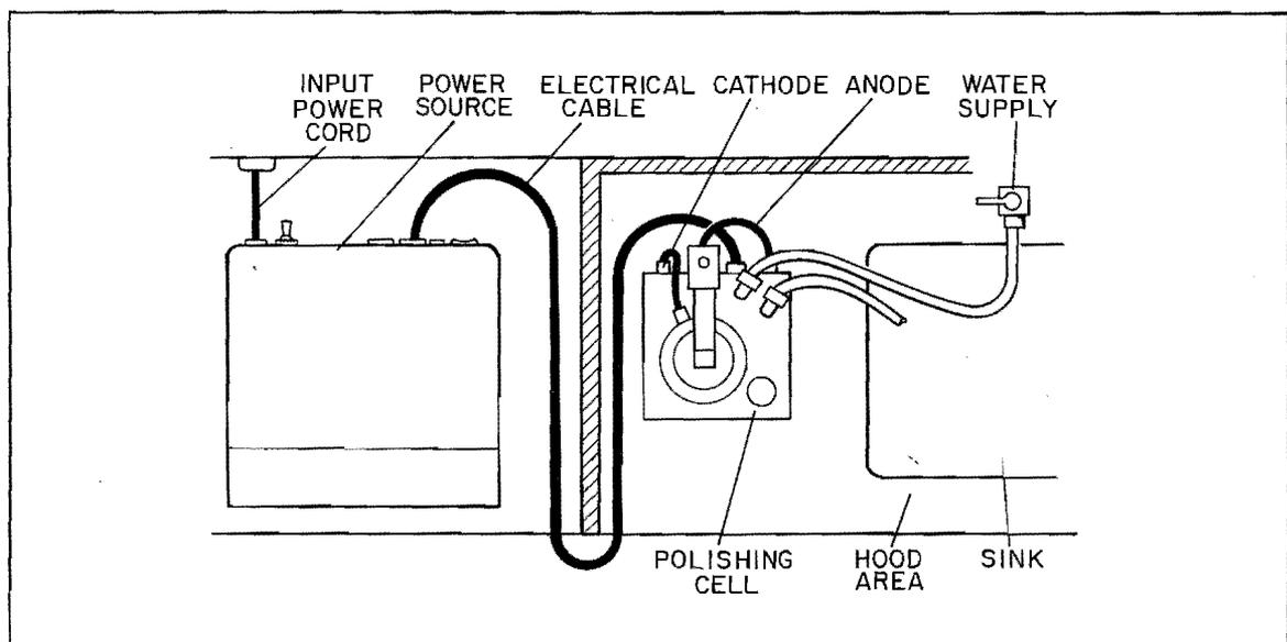
Figure 3. Layout for ELECTROMET<sup>®</sup> 4 Power Source with Polishing Cell (Top View)
