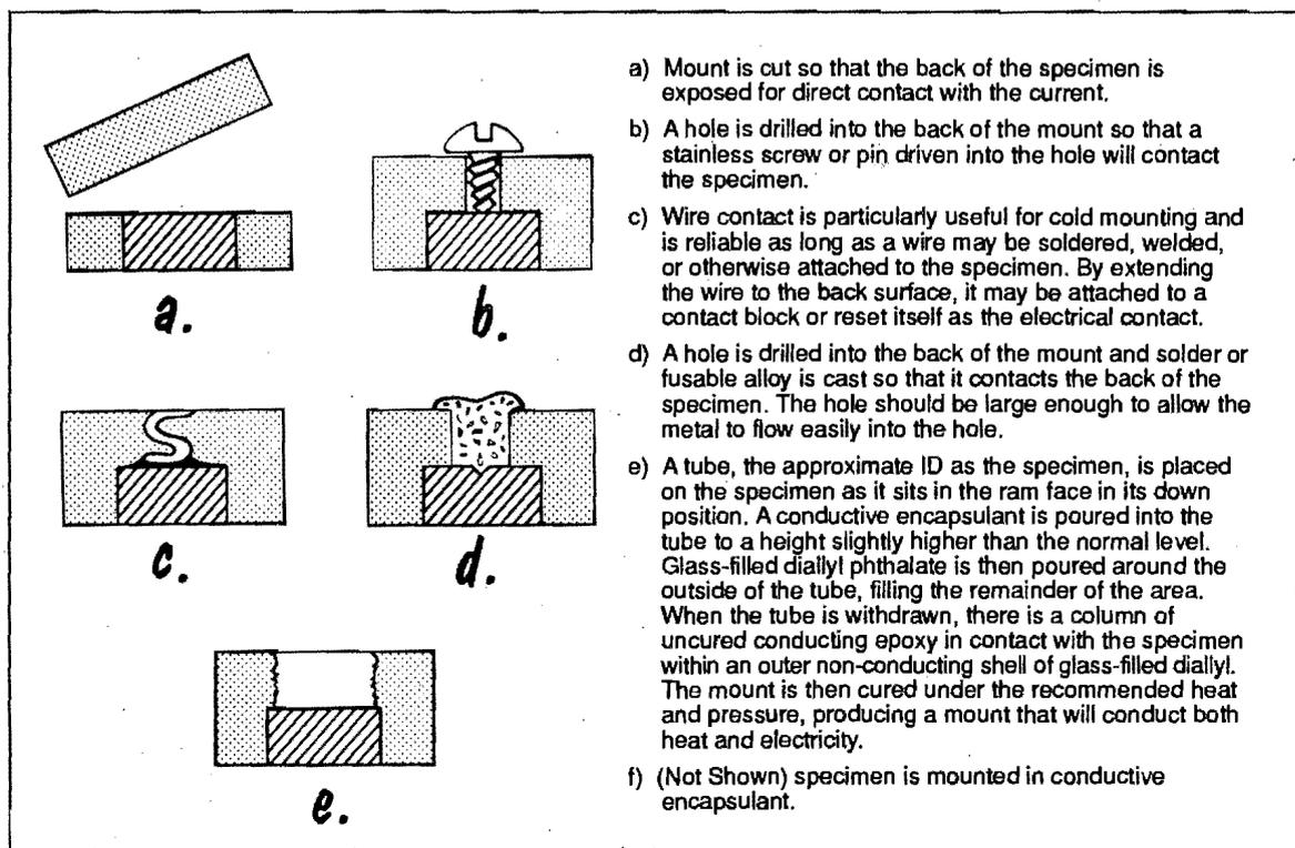
Figure 5. Methods for Making Conductive Mounts
