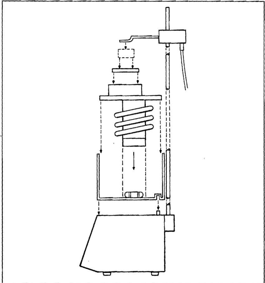
Figure 2. Polishing Cell Installation Detail
