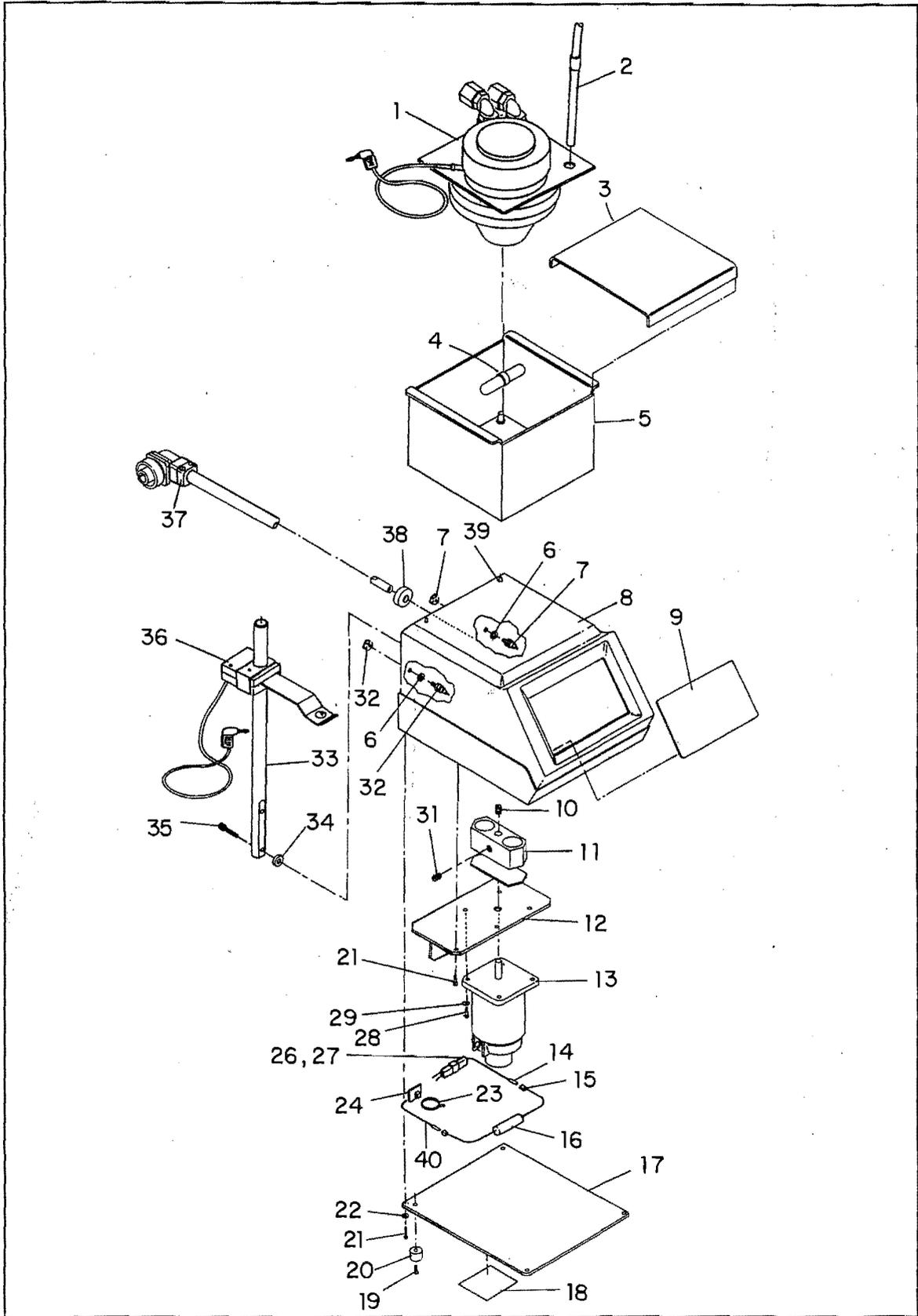
Figure 11. Parts Diagram for ELECTROMET® 4 Polisher/Etcher Polishing Cell
