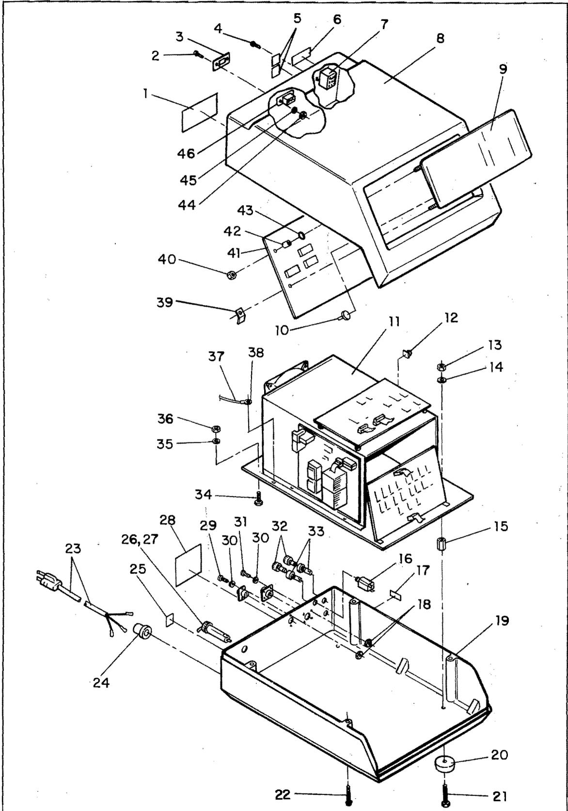
Figure 12. Parts Diagram for ELECTROMET® 4 Polisher/Etcher Power Supply
