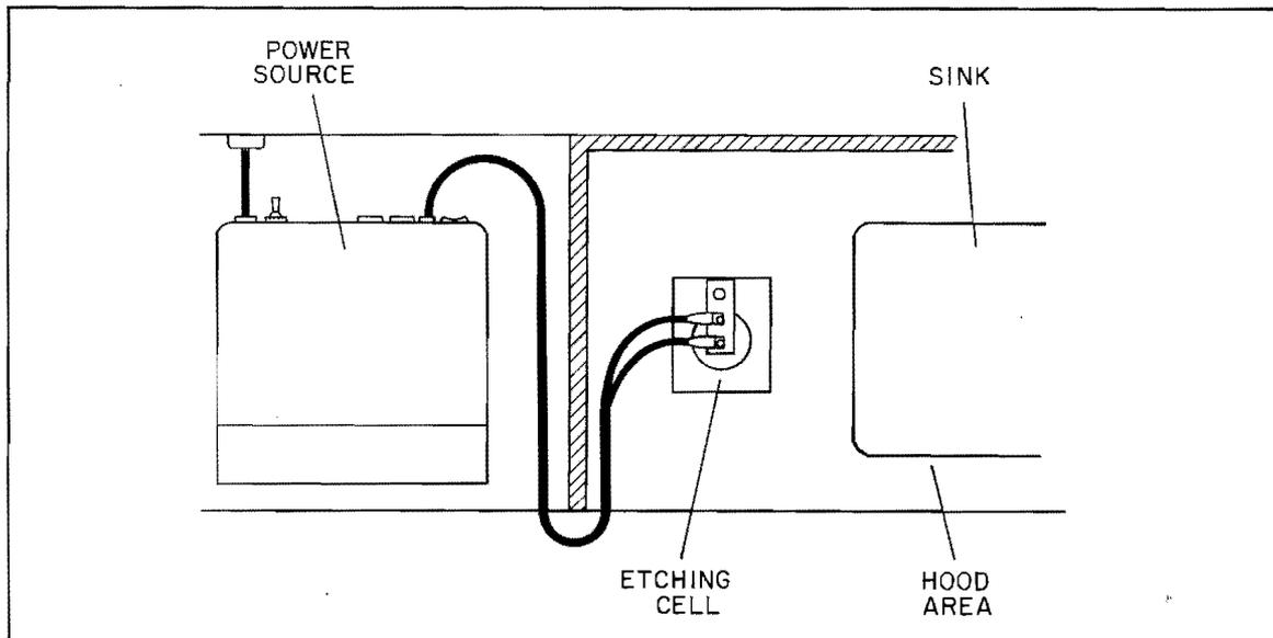
Figure 4. Layout for ELECTROMET® 4 Power Source with Etching Cell (Top View)
