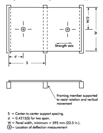
Figure 4. Uniform Load Test Specimen Diagram shows strength axis parallel to supports.
