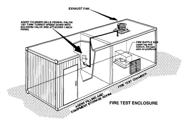
Figure 1. HF and visual obscuration test and evaluation equipment.
