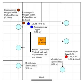
Figure 3. 28 m<sup>3</sup> compartment layout
