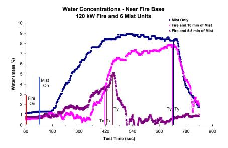
Figure 6. Water mass concentration from several 6 mist unit tests
