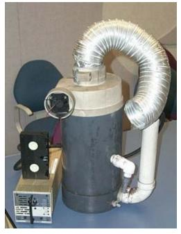
Figure 2. Picture of NanoMist<sup>™</sup> mist generation unit
