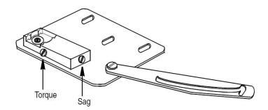
Figure 1. Undercounter Hinge Bracket for Glass Door Adjustments
