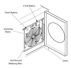
Figure 5. Six Inch Chart Recorder
