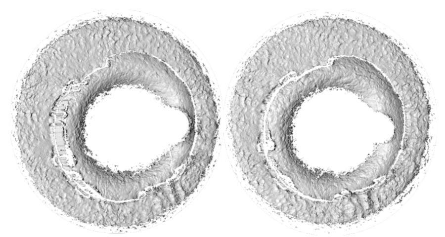
3-D topographic images of breech face impressions obtained from a pair of cartridge cases ejected from the same firearm slide.
