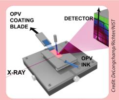
Schematic of real-time experiment, showing custom film coater assembly, incident x-ray beam and imaging detector, and normal incidence optical probe.
