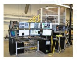
Figure 2. Control-center and overall view of the ARRAfunded, next-generation metal formability system, based on in-situ monitoring of cruciform specimen deformation.
