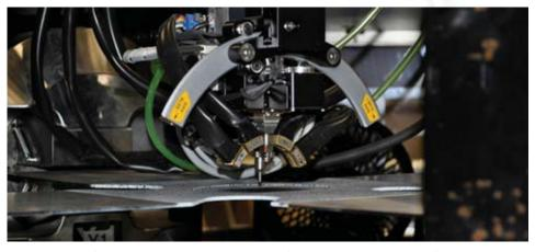
Figure 3. Close-up of x-ray stress measurement mounted on the cruciform system, positioned above a deforming sample
