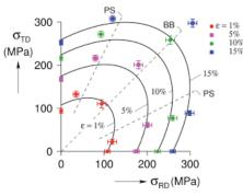
Figure 1. Flow stress of 5754 Al as a function of strain
