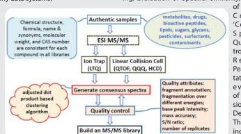
Procedure for building an ESI MS2 library compounds in complex mixtures of non-volatile compounds. The identification step can be aided by matching acquired tandem mass spectra (MS2) against reference library spectra. It has been a significant challenge for the researchers in the NIST Mass Spectral Data Center to generate library quality ESI MS2 data for target analytes due to complex ESI chemistry. Depending on the compound, a
