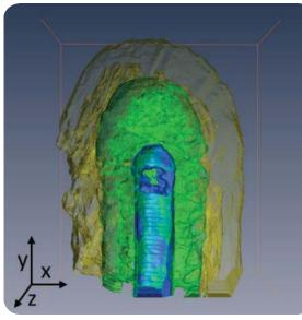
A colorized 3D side view of a battery showing the metallized silicon core and its outer layers. Credit: Oleshko/NIST
