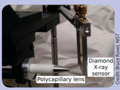
X-ray Absorption Spectroscopy photon delivery system. The polycapillary lens focuses the large X-ray beam to a 30 micron spot at a distance of 6 millimeters. The diamond sensor, in operation, is rotated to a position adjacent to the outlet of the lens, leaving room to place the sample at the focal spot of the X-rays.
