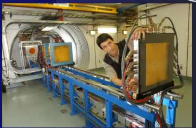
NSRL beam line and target room showing one of the four ion chambers used for beam imaging.
