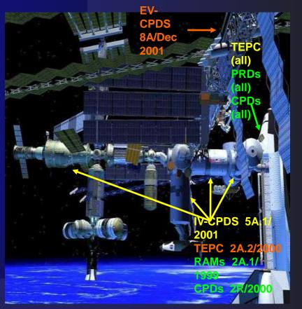
Active instrument real-time telemetry Active instrument no real-time telemetry Passive instrument
